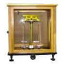
It is of short-armed triangular type beam. It is highly suitable for research work in universities and industrial laboratories specially designed to maintain constant sensitivity under varying load and acute self-acting parallel arrestment of the beam. Capacity 200gm approx. with sensitivity of 0.1mg.
