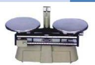
Two pan balance for accurate and rapid weighing up to 2 kg. when used with supplementary masses. The balance has a cast alloy base and featured angled beam with center reading poises, magnetic damping, spring loaded zero adjusted compensator, precision ground knives and cross braced aluminium alloy beam.
