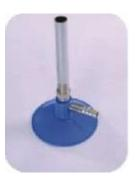
Nickel plated burner tube with rotatable air regulator & Cylindrical riffled connector, mounted on pressed steel base. Burner tube 12.5mm dia, base 75mm, dia overall height 150mm. Connector 10mm O.D. to be used with LPG Gas.
