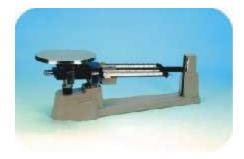
Triple Beam Balance are specially designed to handle weighing solids and powder. Three notched and tiered beams with center reading . Indicating sliding masses giving total weighing capacity of 610 gm. The capacity can be increased up to 2610 gm. by using supplementary masses. Spring loaded zero adjust compensator and magnetic damping are provided for fast setting and reading.
