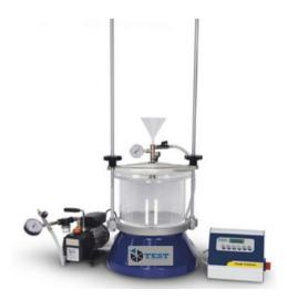
THEORETICAL MAXIMUM SPECIFIC GRAVITY OF UNCOMPACTED BITUMINOUS PAVING MIXTURES (RICE-TEST). Equipment used to perform specific gravity and density measurements on asphalt and other materials.
