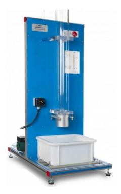
The Drainage Permeameter, "PPD", allows to measure the permeability of different filter materials before the passage of fluids through them, as well as to determine the most optimal combination of filter/soil.
