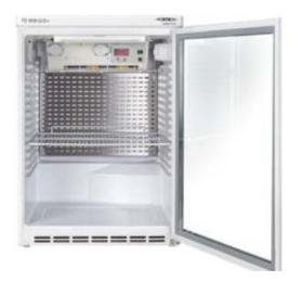
Compact thermostatic cabinet for up two OxiTop® IS 12 stirring platforms. It is easy to integrate into the working environment and perfectly suited for standard applications. It has two internal plugs for connecting stirring platforms.
