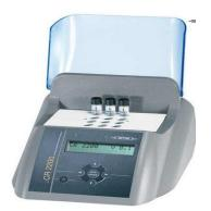
Equipment used to perform COD measurements.
