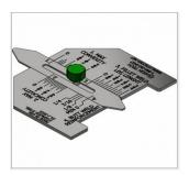
Imperial welding gage TWG-2 (also known as automatic weld size weld gauge) to be used for: checking reinforcement, checking the throat of fillet weld and determining the leg size of the fillet weld.
