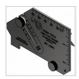
Welding gage TWG-1 (also known as bridgecam or cam type) for measuring in either inches or millimeters the following: angle of preparation, excess weld metal, depth of undercut, depth of pitting, weld throat size, and more.
