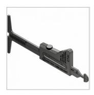
Welding gage TWG-6 (also known as hi-lo) for measuring interior misalignment, pipe wall thickness, bevel angle, fit-up gap, fillet leg lenght, crown height, fillet weld size and for preparing socket welds.
